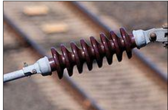
Fig. 2. Insulator used in electrified railways (1).
