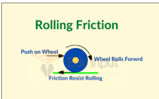
Figure 3. Rolling friction due to the forwards rolling of the wheel (2).
