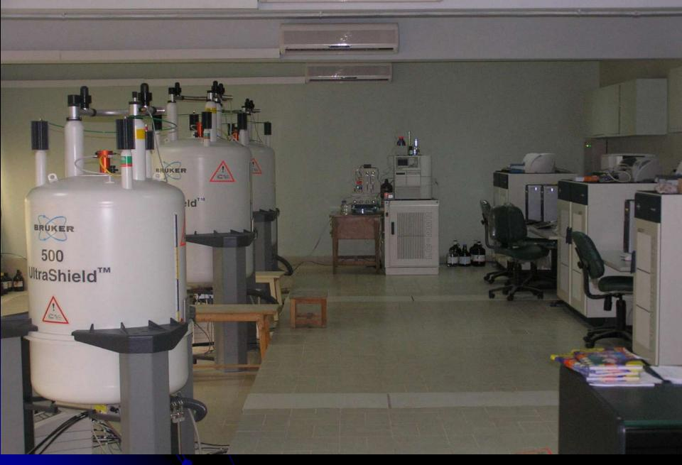
NUCLEAR MAGNETIC RESONANCE SPECTROMETERS
